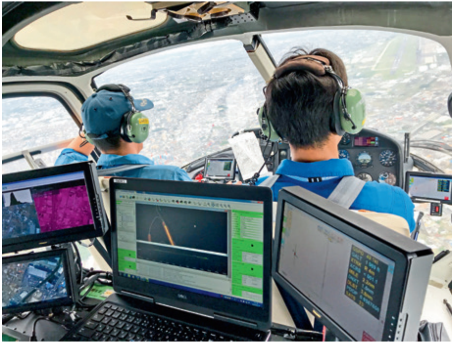
All monitors and controls are put together in a compact console. The operator shares flight guidance with the pilot via two monitors mounted in the cockpit
